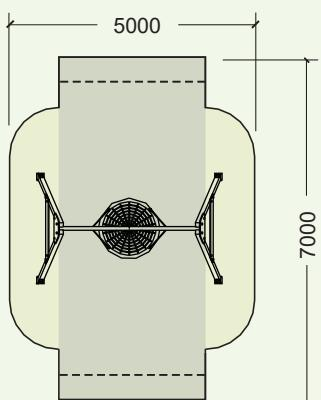
The shaded area requires impact attenuating surfacing. The length of this area can be reduced by 0,50m at each extreme in case of using synthetic safety surface.
